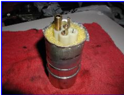
Now the foam with the smaller pump is inserted into the canister.
