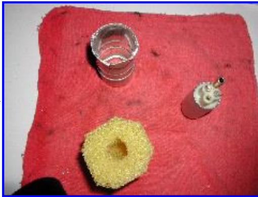
The old BMW fuel pump outer canister, the NAPA fuel pump, and a piece of foam I cut out of the large block.
