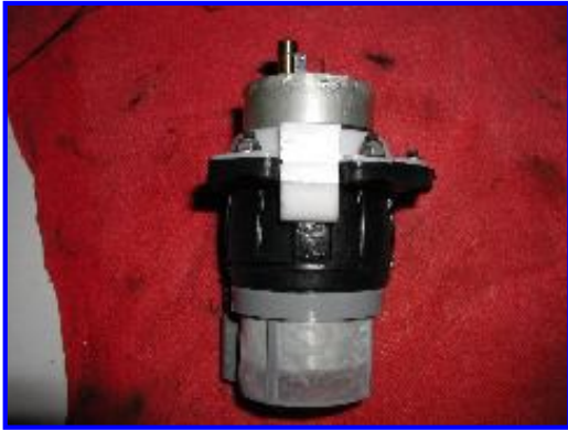
The BMW fuel screen fits perfectly onto the bottom of the canister.
