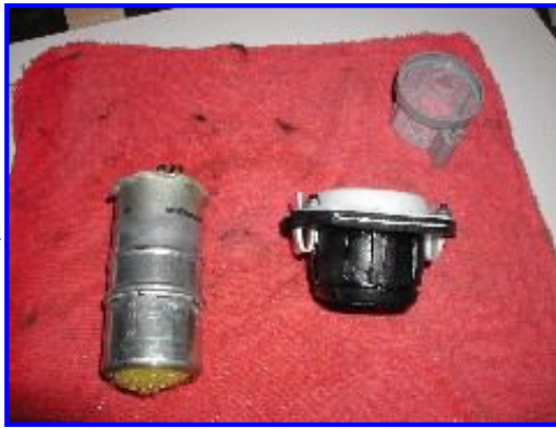
Now the old canister will fit perfectly into the BMW gasket.
