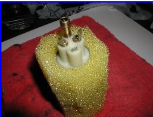
The new smaller fuel pump is inserted into the foam.
