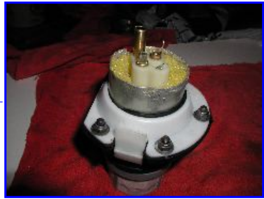
The entire assembly is ready to snap into the bracket inside the gas tank.
