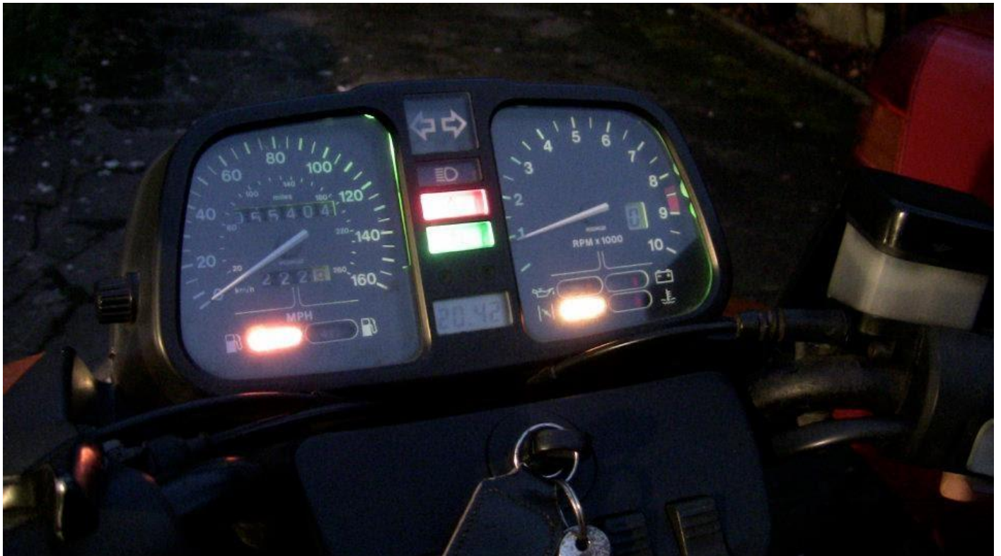
The original dials used to let in water so I swapped them out for an Acewell.
